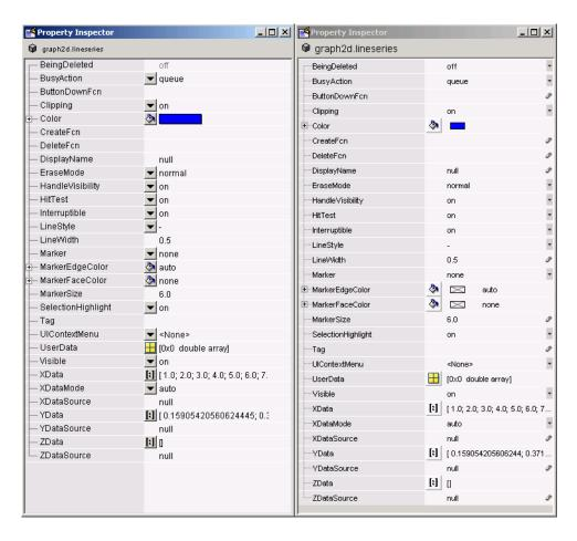
Note that in addition to having a smaller font and wider line spacing, the new inspector locates pop-up menus at the right margin instead of between the two columns. Also, some icons have been redesigned.
